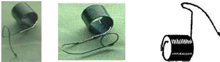
Hooks: There are many different types of hooks as well. Here are just some sample hooks. The point of the hook is always the sharp pointed item that the thread is picked up by, and then later let go of as it has passed around the bobbin case.
