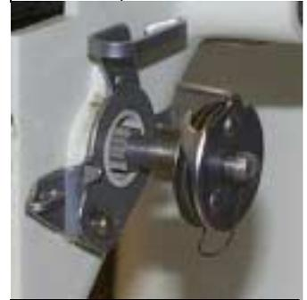
Assemble the unit in your hand, and then slide onto the Stud. Face Check Spring downward, and slide all the way into place.
