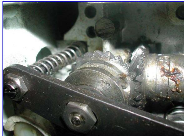
One can improvise a depth gauge, as long as you measure from the top of the hook to the base of the hook driver (winder), shown below, white arrow
