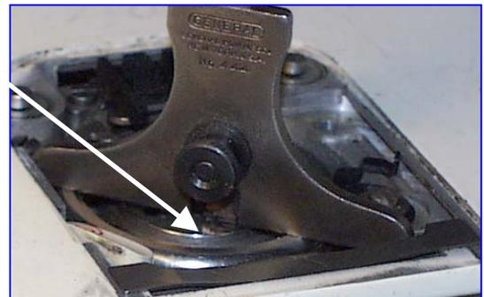
Other fine-tuning is available on the 600E, and this can be achieved by utilizing the two lock screws
